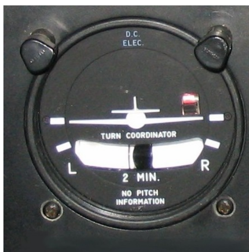
Figure 5.1: A real turn coordinator face. The miniature airplane banks to show roll and turn rate; the doghouse marks show where to level the wings for a standard rate turn.
