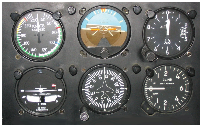
Figure 1.1: A real six-pack panel in the basic T. The attitude indicator sits at the crossing point, airspeed to its left, altitude to its right, heading directly below.
