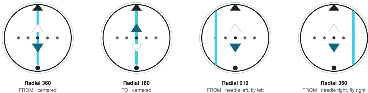
Figure 6.2: Four CDI readings, all with course 360 selected. Only the aircraft's actual radial changes between them.
